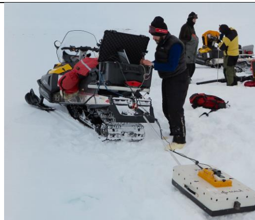
Setting up the GPR on a snowmobile to profile lake-bottom sediments
